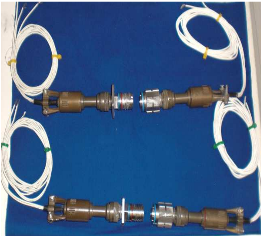
Filtered Harness Assemblies Prior to Salt Fog testing at Environmental Associates
